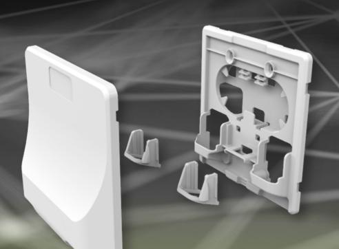
The Connect Terminal is an indoor, customer wall outlet that is designed to fit any 4x4 surface wall box. It allows for splicing of 2 fibres and can fit 1 x SC simplex (LC duplex) adaptor. In addition, the Connect Terminal houses two ports for either 2 x coaxial cables or 2 x LAN cables or a combination of both.
